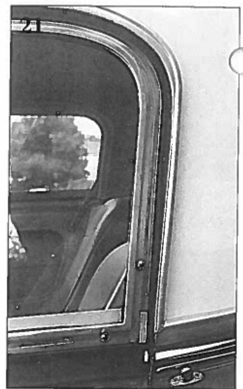
Photo 19: Wrap a small ring of clay around the screw that attaches the top of the rear window braces. This seals out water. Photo 20: When mounting the hardtop, position the hold-down J hooks so that they do not touch the cockpit surround aluminum. Careful positioning of the hood will allow the wing nut to just clear the trim material when tightened. Photo 21: Correct fit shows a uniform gap between the side curtain and cant rail. Still, the hardtop rides somewhat high at the corner against the cockpit surround. This space is filled by the thick rubber block at these corners.
