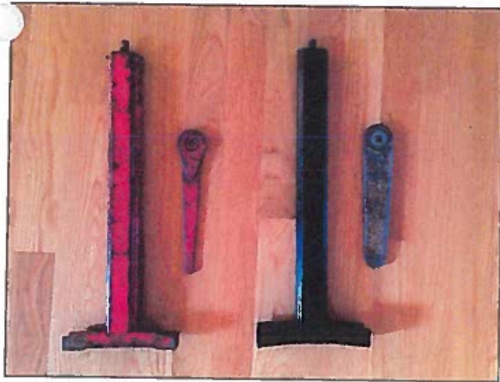
Figure 5. Jacks found in late Mark II, Mark III, and Mark IV Sprites.
