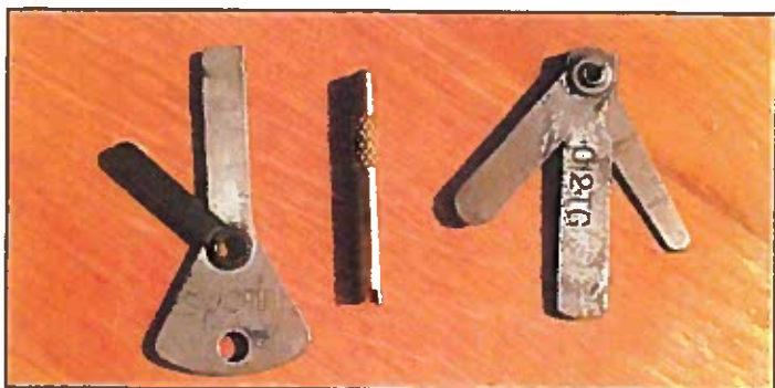
Figure 2. Screwdriver and gauge - Ignition, Spanner - Tyre Valve, Gauge - Feeler - Tappet and Sparking Plug.
