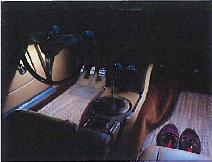
Cockpit Lighting is produced by LED Strips located under the Dash Panel. All of the Interior LEDs are switched by means of the Panel Lighting toggle
