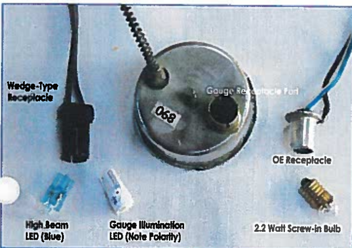
The original and replacement bulbs plus typical receptacles for gauge lighting.
