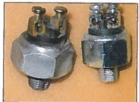
Replacement switches (right) have a slightly smaller hex size than the originals. They come in two "flavors" – a) with screw terminals for earlier cars and b) with blades for push-on connectors (not shown here) found on later cars, starting during 3000 production.
