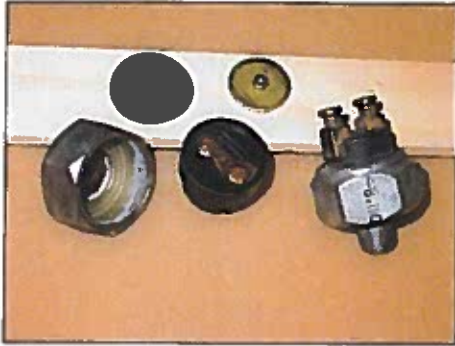
Right – an original stop light switch. The case on the left has had the rolled lip that retains the Bakelite base machined away. The switch nipple is tapered, with 27 threads per inch (American Standard Taper Pipe Thread).
