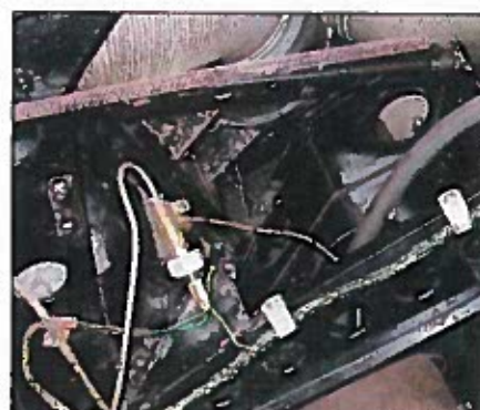
Location of the brake light switch on BJ8s. In this photo the horns have been removed from the riser. This is an original switch with the push-on electrical connections.
