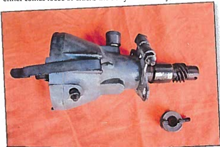
▲ The drive from your old pre-BJ8 six-cylinder distributor can replace the little drive on the Pertronix distributor.
