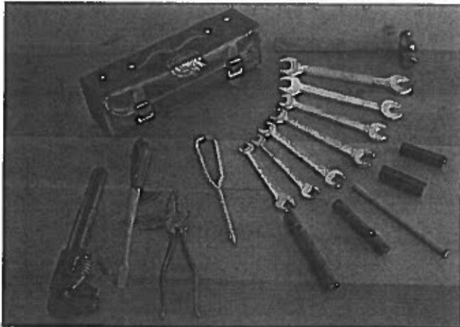
Photo 9 - Only the hex drain plug tools and hold-all box in this photo of a 97H 2100 are reproductions. Because of the weight of the tools I concluded that the box must have had a structural liner, which I made from 1/8-inch cardboard, similar to that found in trim board applications. The covering is original British tool roll material, with a silk-screened BMC rosette. All dimensions were scaled from the tools in the original photo.
