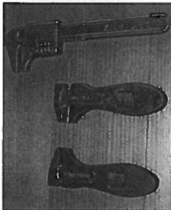
Photo 10 - Tool kits found in production 100s built in 1953 and as late as March, 1954 came with Hubert grease gun (top), kits in cars from June, 1954 on had Verulam 2788 ones. Both versions came with an adapter nozzle for filling the steering box with oil.
