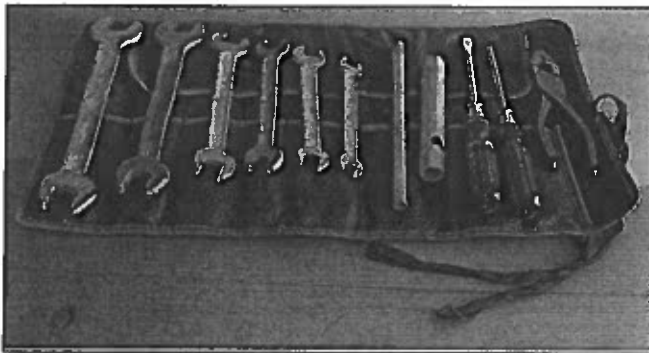
Photo 6 - An original AKF 1596 tool kit. Box spanners have been seen mostly with zinc-plated finishes, though a black oxide finish is also possible.
