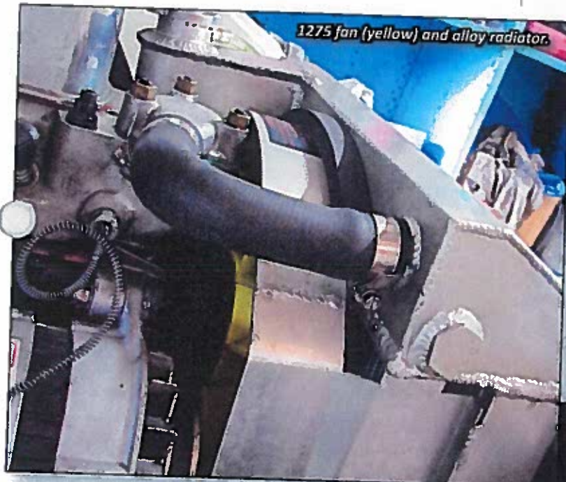
A bespoke shroud on 100 (the flat panel behind the air duct and taped wiring).
