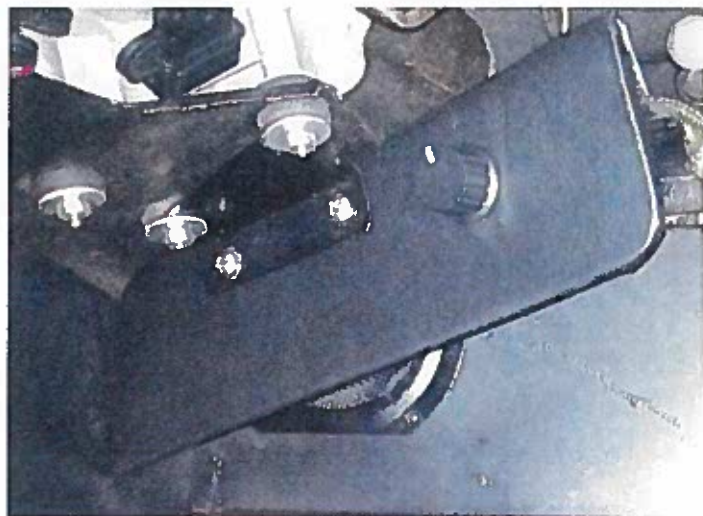
Fig. 5 - Drivers Foot Well - Deflector Only
