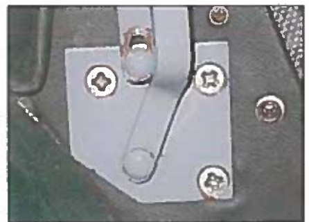
Photo 14 - This photo shows the second style of top frame mounting plate. Note the male snap at the right that a flap on the top will attach to. The mounting plate of the first style had a slight peak at the center of the top edge, instead of being straight. Otherwise the top bows are identical.
