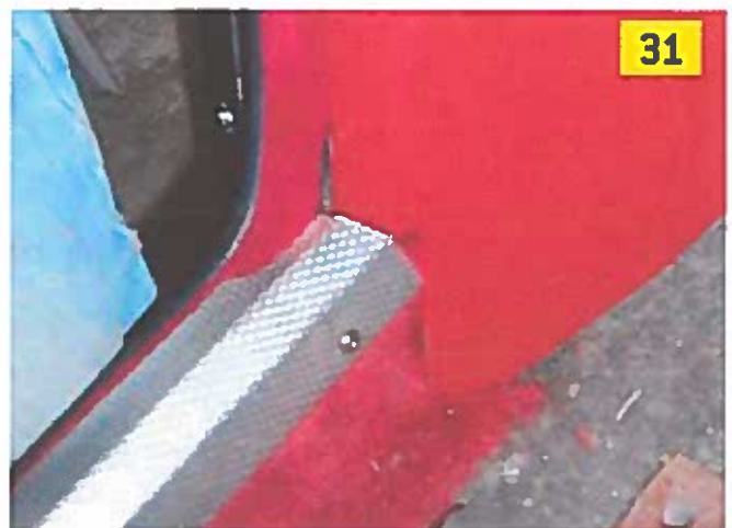
Photo 31: The sill plate covers most of the seal furlflex.
