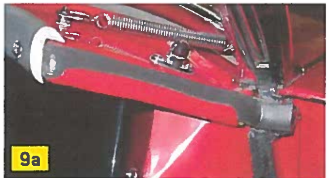
Photo 9a: BN1 scuttle seals are nested into a channel formed into the edge of the scuttle area of the aluminum front shroud and glued to the flat face. The rear end is shaved to about half-thickness, tucked behind the cockpit molding for about 1.5 inches and is held in place with a trim screw (as in Photo 2). The forward end is glued against the rear face of the windshield stanchion. Note that this part of the stanchion is painted body color.
