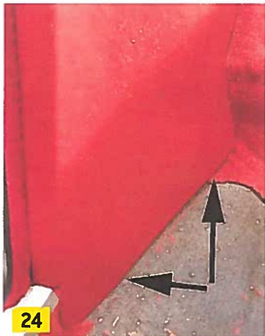
Photo 24. The edge of the rear carpet (about 1/2 inch or so) needs to be able to tuck under the panel. This photo was taken after attaching the seal strip and sill cover plate.
