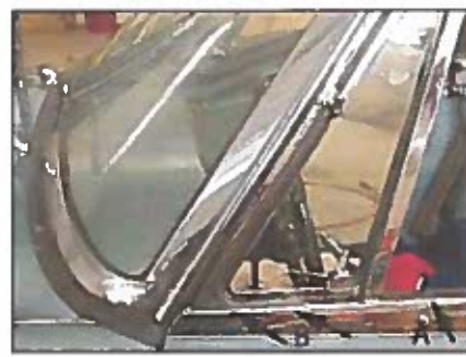
Photo 10 - The outer sweep seal [A] is mounted to the chrome trim piece before installing on the door. The lower vent window frame seal edge is trapped behind the chrome trim [B].
