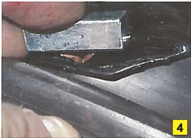
Photo 4: Insert the split rivet through the washer, flap and flange hole and, while holding it up firmly with a blunt tool, pull back the top part of the seal and use a flat-blade screwdriver to partially open the rivet tips. Then, still holding the seal bent back, place a small square metal block across the rivet tips as shown.
