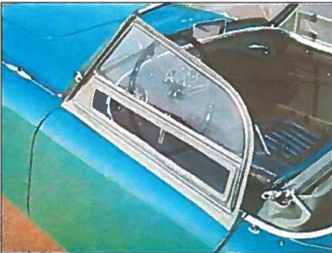
Photo 5a - The second style of side curtain for the 100 had a leathercloth and flexible plastic cover attached to a metal frame. Slotted brackets at the bottom edge of the frame allowed ample adjustability. The lower rectangular flap lifts to provide access to the interior door latch.
