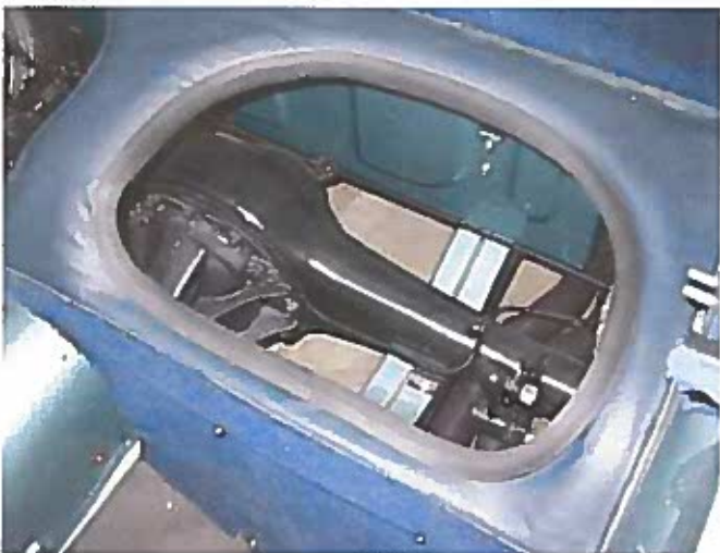
Photo 4: A seat pan seal installed on a BJB. The appearance is almost exactly like the original.
