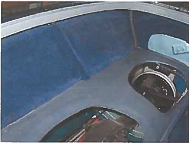
Photo 3: The rear cockpit area of a BJB. The thin foam padding under the vinyl should be cut back from the edge of the seat pan openings and where the wheel arches meet the shelf. The vinyl should be glued to the painted metal lip around this edge, but not to the foam pad.
