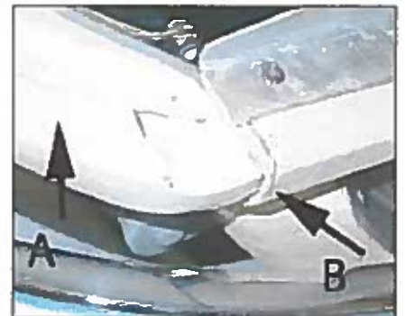
Photo 24 - The trimmed front wood block (A) is screwed to the header bow. Note how the side block trim meets to form a tight edge joint (B).
