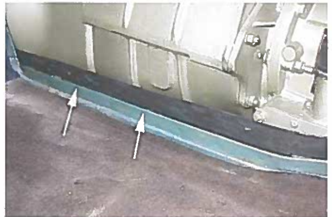
Photo 20: To replicate the original inverted "J" seal, first glue the 1/8 inch thick foam strip to the back side of the metal flange, leaving enough projecting up to reach down to the floor on the front face.
