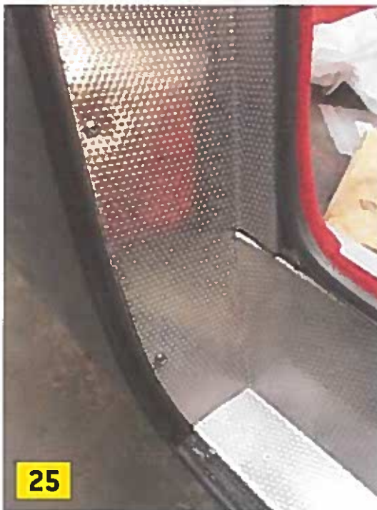
Photo 25: The vertical door pillar facing slides in behind the sill piece. Shims are often needed to hold the shut facing tight against the rear sill edge. The piping ends at the rear corner of the horizontal sill.
