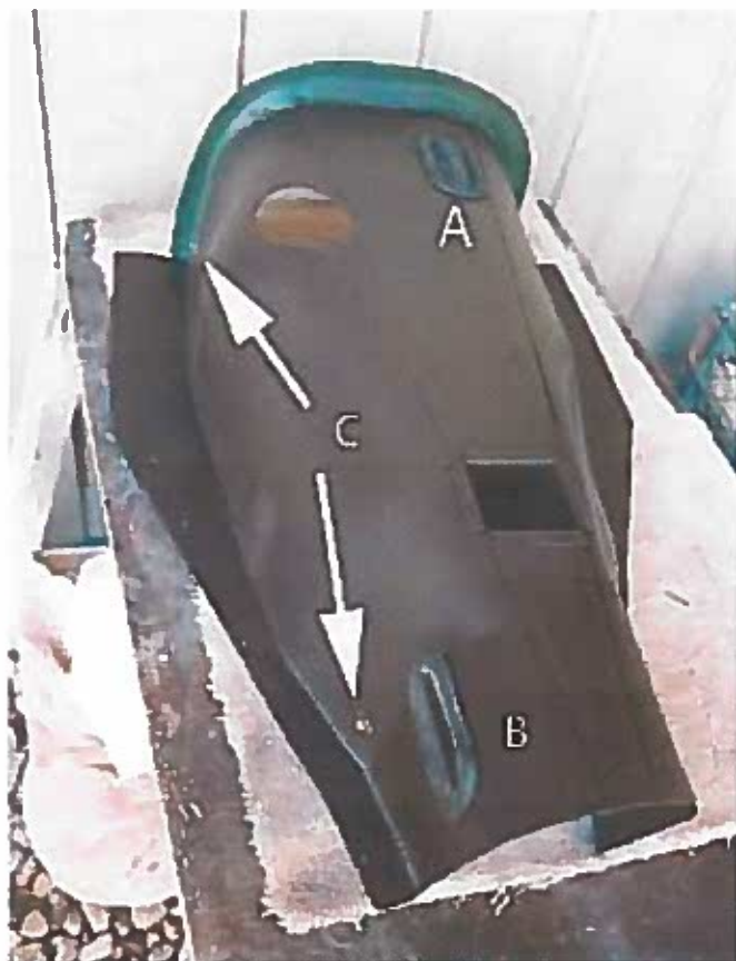
Photo 14: This is the style of gearbox cover used on all 100-Six and 3000 roadsters (up to the center-change gearbox). The 6-cylinder roadster cover had two longitudinal seams, as compared to the single seam on the BN2 cover. The front flange was wider (shown here) on 3000s than on 100-Sixes. On cars with grey interior trim, carpet binding around the gear lever and handbrake was done in grey vinyl, as was the piece glued behind the brake handle and the front flange was trimmed in either green (shown here) or red to blend with the carpet. On all other trim colors (black, red, or blue), the front flange trim as well as all carpet trim and binding was the same vinyl color used throughout the interior. The rubber gear lever gaiter is shaped on the underside to fit snugly over the metal gear lever retaining cup on the transmission (see also Photo 10). Rectangular ports with rubber plugs provided access for filling the gearbox (A) or lubricating the forward driveline grease fittings (B). As with the BN2, the gearbox carpet was attached using snaps (C).
