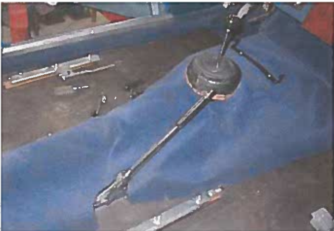
Photo 23: Gearbox carpet cover—the raised fiberglass dome has its original vinyl covering. On Mk II roadsters and BJ7s this “tower” was covered in the same color vinyl used for interior trim. The covering was black on all BJ8s, as shown here, regardless of interior trim color. The baggy fit of the carpet can also be seen in period factory photos. On BJ8s there was no rolled edging around the handbrake cut-away. The black bracket in front of the gear lever is for fixing the console. On LHD cars the left-front of the carpet must be folded back to gain access to the gearbox dip stick, so the speedometer cable feeds under the front part of the carpet and exits at the top edge.
