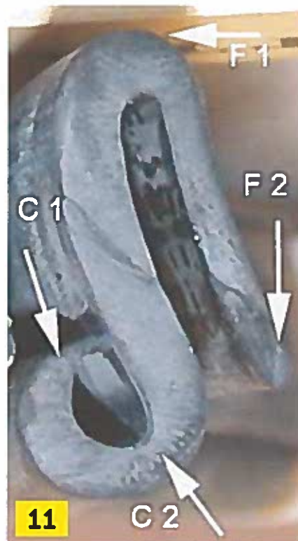
Photo 9b: This skinned foam extrusion is an excellent approximation of the original BN1 scuttle seal. The flat face that is down in the photo mates against the metal scuttle. I find that by only applying adhesive along the bottom half of the back surface, the seal will stay in place but is still easy to replace when needed.
