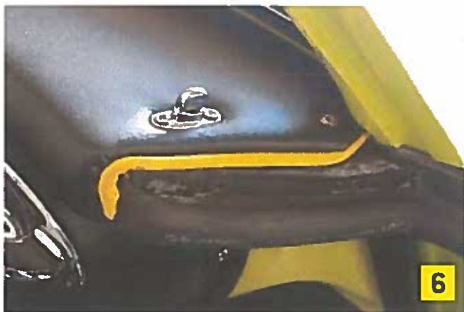
Photo 6: Note the trim screw and cup washer at the front corner of the dash pad. Access to this screw is blocked by the windshield pillar. On a number of original roadsters (3000 Mk Is) this screw had a flat (rather than raised) Phillips head, and was chrome plated like the regular trim screws.
