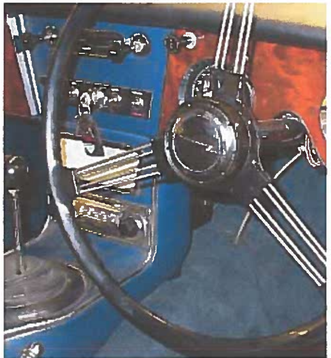
Photo 25: This photo of a totally original BJB with 16,184 mi. on the “clock” (built October 13, 1967) shows many details. 1) There is a strip of matching piping attached (with “D” clips) along the top edge of the console where it meets the bottom of the dash. 2) Around the gear lever the narrow edge of the stainless trim should show. 3) On this RHD car the speedometer cable pokes through a hole in the carpet. This cable would be shorter than on a LHD car and exit through an appropriately-located hole in the gearbox cover. Since access to the gearbox dip stick is on the left side, this doesn't interfere with folding the carpet back. 4) This car has non-adjustable steering -- thus the larger horn button and different switch bezel design.
