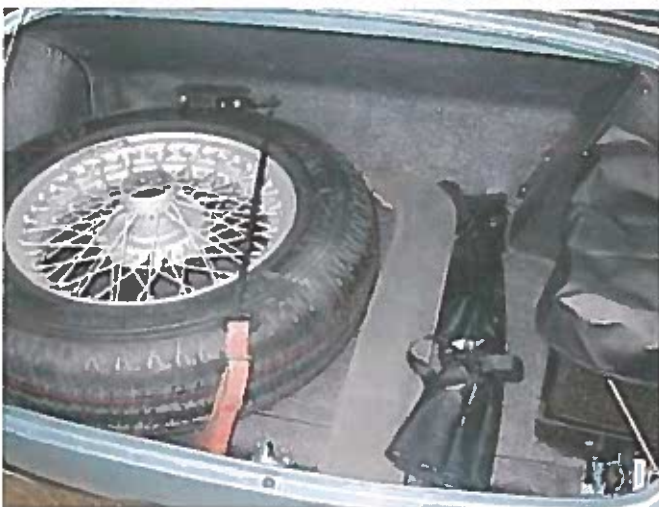
Photo 1: This photo shows how a completed BJB boot looks, with tool kit, tonneau cover support bar in its Armacord case, tire hold-down equipment, and plastic battery cover. Boots of earlier 3000 series are virtually identical.
