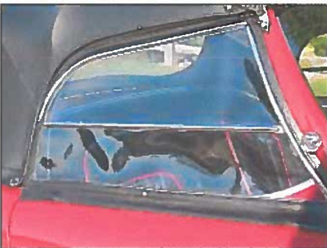
Photo 5b - The third side curtain style used on 100s was very similar to the second one. In this case, the lower rear corner lifts outward to create access to the interior.
