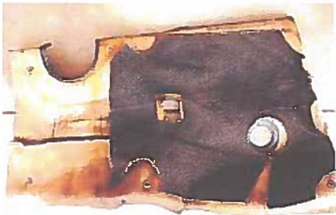
Photo 15: This photo shows the jute pad glued to the underside of an original BN6 gearbox carpet. The carpet extends all the way back to the rear bulkhead and now has a wrapped vinyl binding around the opening to clear the hand brake.
