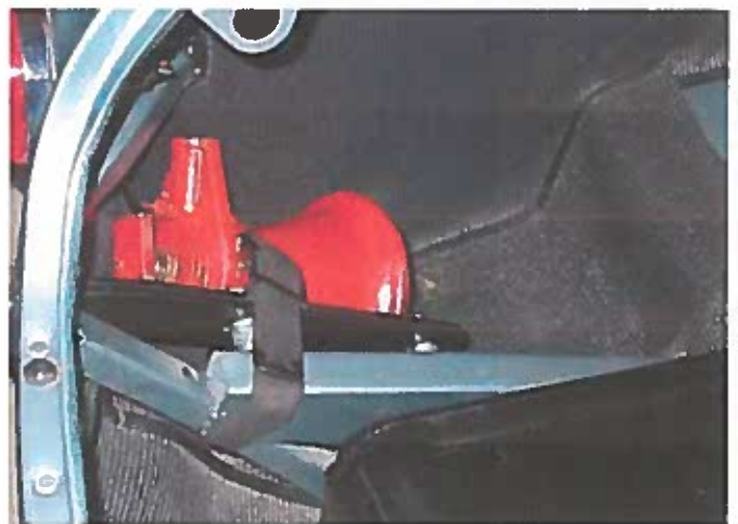
Photo 2: Starting with 3000 MkI BN7 C.10611 and BT7 C.10565 (around summer, 1960) the black King Dick B.1881 jack was replaced with a shorter Chinese Red Shelley LJ225 one with a conical base. At this point a strap was also included for securing the jack against the left rear bumper bracket. This photo is of a BJB. Note the reinforced lip around the nose of the jack where the handle inserts. This design change occurred early on during BJB production to correct a problem of the yoke pocket breaking.
