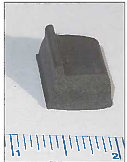
Photo 13 - An excellent seal that is almost exactly like the original one is available from Restoration Specialties ( www.restortionspecialties.com ) -- their item number 4116. The left face in this photo nests against the inside of the front bow angle (see area "C" in Photo 12).
