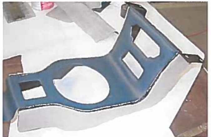
Photo 24: Thin foam padding was used on the console sides and on the vertical face of the console. There was no padding on the horizontal surface. Joints between the side and top vinyl pieces must be tight and precisely aligned so they will be hidden by the narrow stainless trim strips. The foam padding needs to be cut back slightly near the trim strip so the vinyl coverings can be glued to the metal console surface.
