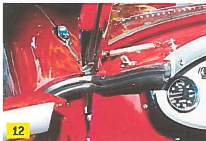
Photo 12 BN2 scuttle seals are mounted using two additional steel pieces. The narrow metal strip clamps the back flap of the seal against the hinge pillar bracket and the angled scuttle edge. The seal flap at the rear is also held behind the cockpit molding by a trim screw. The lower windshield stanchion and fixing bolts (below the seal) should be painted body color, as is done on BN1s.
