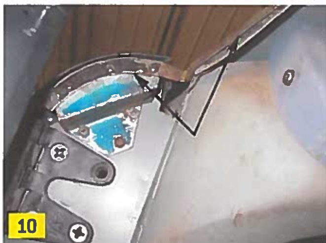
Photo 10: This view shows the metal pieces used for mounting the BN2 scuttle seal. The thin securing strip (arrows) nests into a slot in the rubber seal and is shown here to illustrate how it will be mounted. Note the screws attaching the fan-shaped bracket to the hinge pillar are larger than those for the securing strip. Three screws are also used to fix the straight part of the strip against the scuttle.
