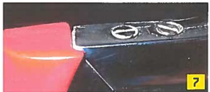
Photo 7: Only the top corner bracket screws are visible so save those with the nicest finish for these locations. The chrome channel faces at each mitered corner should be flat right up to the joint. Over-polishing will round the edges of these soft brass pieces.
