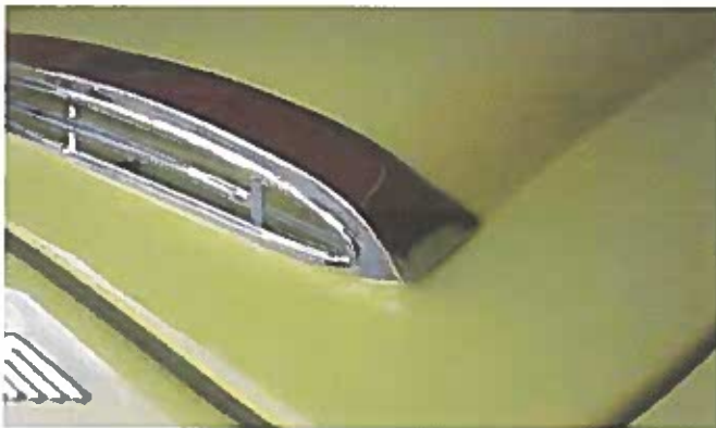
Photo 8: The end corners of the brow typically do not line up perfectly parallel with the creases on either side of the bonnet scoop. You may well have to live with a less-than-perfect fit between the chrome brow ends and bonnet surface. Be particularly attentive to possible gouging of the paint by the brow. Being brass, it is fairly soft and easy to reshape a bit by twisting gently.
