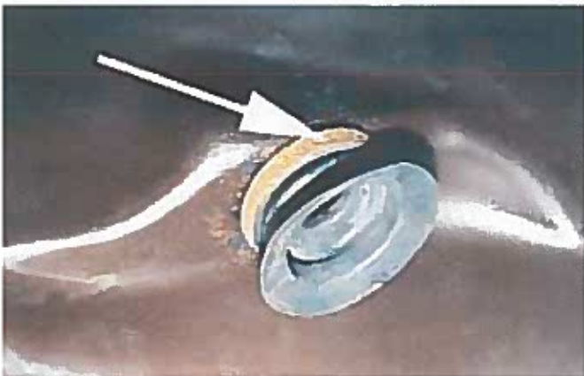
Photo 9: A 3 1/2 inch diameter by 3/8 inch thick skinned foam donut (arrow) fits into the top groove of the gearshift boot before inserting the boot through the gearbox cover hole. The cylindrical cavity in the bottom of the boot will nest over the gear lever cup on the transmission. The underside of the aluminum cover is finished in a dark brown primer.
