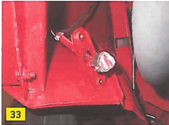
Photo 33: The far end of the wire has a loop formed to accept a 10-32 screw. From under the car, you can reach over the front of the sill structure to pull this loop out where the check strap can be attached. Note the orientation of the tang curvature relative to the off-set hole in the plate. Tighten the screw with the tang in line with the wire.
