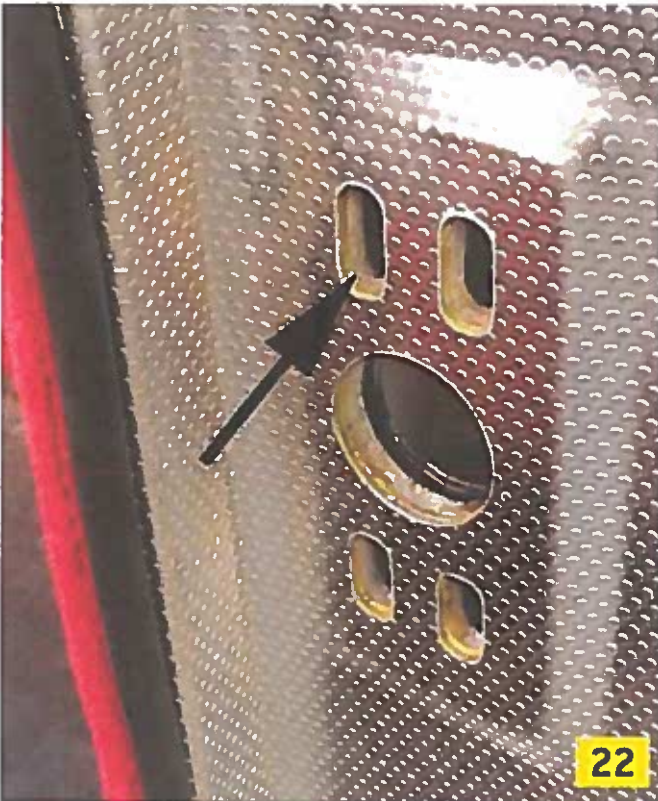
Photo 22: Packing shims (arrow) can be glued to the Al facing to hold them in place until the striker plates are mounted. The number and thickness of these should have been determined earlier while fitting body panels (see Part 20, May 2008).
