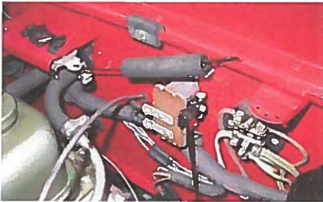
Photo 9: The latch return spring has been unhooked on this Healey 100 and next will be detached from the latch bar and removed so that it won't interfere with closing the bonnet.
