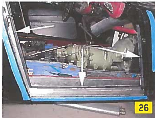
Photo 26: Arrows point to the three door seal sections on early BN4s. The rubber seals slide into metal strip channels and are mitered at the corners. The top edge of the longitudinal aluminum sill trim folds over the sill carpet (not yet installed in this photo), as on 100s. There is no third piece mounted along the inside as on BN6s, later BN4s, and 3000s. Blue masking tape is being used to protect the paint along all edges. In this photo the engine and gearbox have already been installed.
