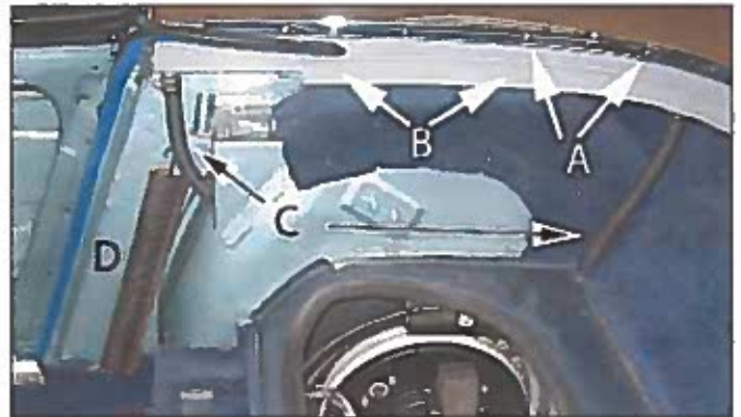
Photo 1 - The drip channel is painted gray and nests under, and behind, the shroud lip. Chrome raised head Pozidriv sheet metal screws (A) thread into the top edge of the channel. Note holes (B) on the channel face. These are for attaching the inverted "J" piece for retaining the rear edge of the top. Drain tubes (C) from the drip channel, and top mechanism springs, and their Armacord sleeves (D), should also be installed now. This photo was taken at a later stage after more of the rear trimming had been done.
