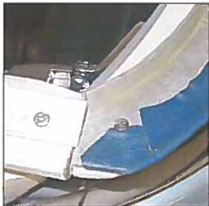
Photo 25 - An aluminum facing is trimmed with top material and screwed to the header bow's wood block.
