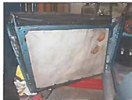
Photo 31 - There is a thin vinyl cover glued to the frame all-around making an air-tight seal to the inside of the door before attaching the trim panel. The foam rubber "donuts" (original ones shown here) push firmly against the panel (and in doing so also make the handles more difficult to install).
