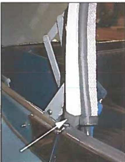
Photo 30 - A filler (arrow) made from foam rubber is glued and screwed to the end of the trimmed wood block. The screw is a Pozidriv trim screw with cup washer and it and the washer are buried a bit into the rubber block.
