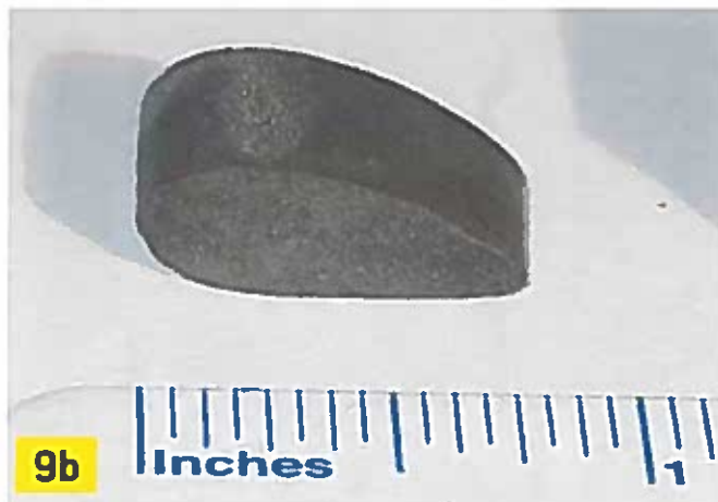
Photo 9b: This skinned foam extrusion is an excellent approximation of the original BN1 scuttle seal. The flat face that is down in the photo mates against the metal scuttle. I find that by only applying adhesive along the bottom half of the back surface, the seal will stay in place but is still easy to replace when needed.
