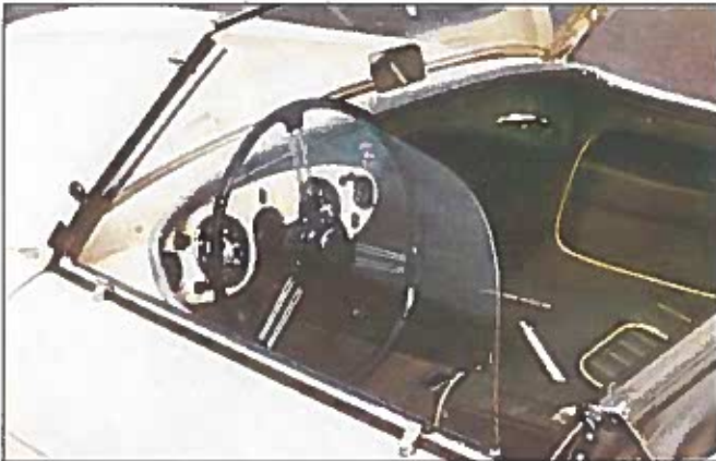
Photo 4 - The window of this early 100 side curtain doesn't show up very well in the photo because the plastic is quite clear. The frame is shaped to match the side curve of the windshield pillar. Mounting pins are non-adjustable on this side curtain design.
