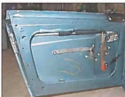
Photo 8 - Two screws near the bottom of the window track [arrow] allow for some positioning adjustment of the vent window frame. The yellow "79" is a copy of the original cayron marking made at the factory. When the vent frame was restored the variety of finishes found on the original was carefully duplicated, including the red primer near the bottom attaching bracket.
