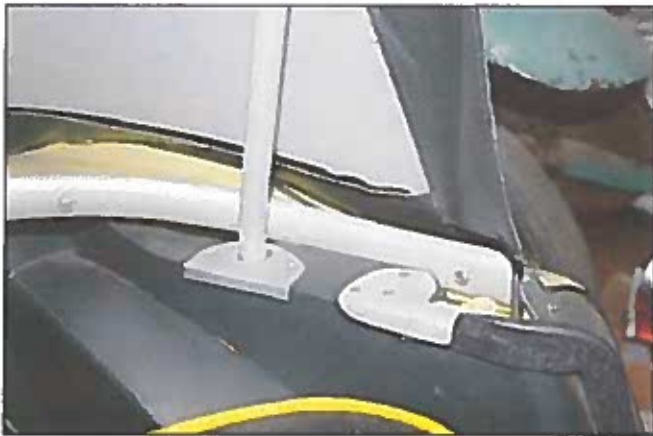
Photo 19 - On BN6 and BN7 Healeys the main frame pocket has a separate aluminum trim piece screwed to the rear quarter trim panel.
