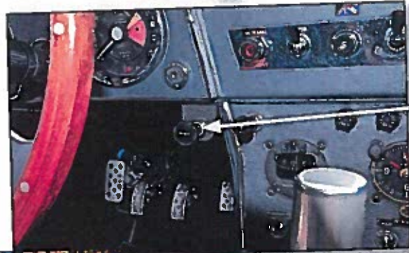
One of many mods to Gary's Healey, this PUSH knob opens and closes the scuttle vent.
