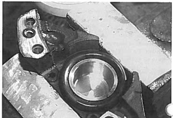
A restored caliper half with fitted with new seals and a stainless steel piston. Note the small, correct rectangular-section O-ring (flat like metal washer) at top left
