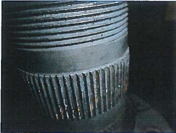
An old hub cleaned to show splines worn sharp at top, wear in the face of the spline, wear in the threads.
