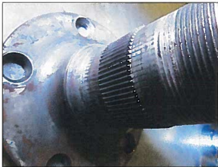
Damage to splines and threads, vertical lines worn into hub.
