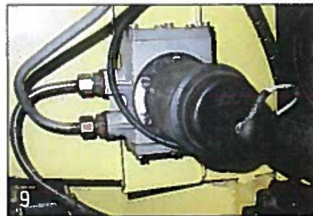
Photo 5 -- The AUA 56 pump was mounted to a shallow bracket using 1/4 BSF x 1/2 inch long hex screws. This bracket mounts to the rear axle side of the heel board behind the left seat.
