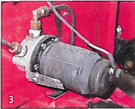
Photo 3 – Installation of the AUA 36 pump on a 1955 BN1.
