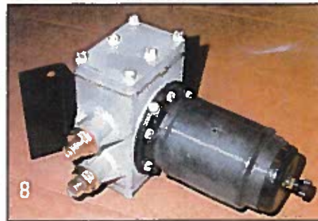
Photo 8 – Inlet and outlet fuel lines were attached using union fittings (brass in this photo). Use of the rubber boot/sleeve was continued from the earlier AUA 36 and AUA 56 pumps.
