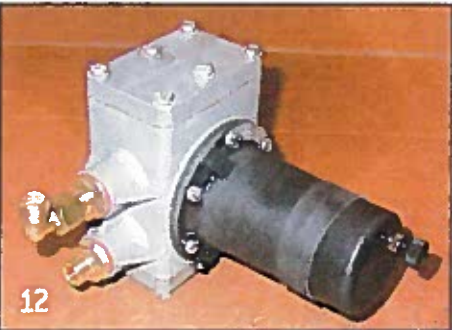
Photo 12 - AUA 172 pump as configured for Mk II BN7s starting at C. 17547 (Jan. '62). It uses the same right angle output fitting as on BN6 pumps. Rubber band replaced the boot cover at Mk I BN7 C.10842 (Jun. '60).
