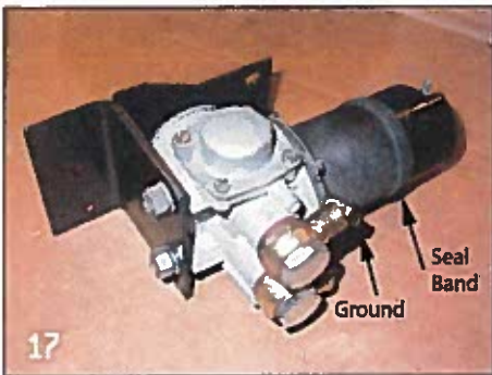
Photo 17 – AUF 301 pump fitted to Phase 2 BJ8s from C.28225 (Aug. '64) to the end of production. It uses the same mounting bracket and banjo fuel line fittings as with the AUA 173 pump. A spade terminal for the ground wire was mounted by a screw into the side of the coil base flange (see also Photo 18).
