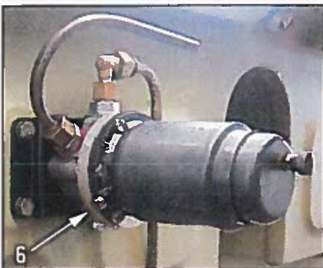
Photo 6– The fuel line segments in this photo have been cut from original lines but show the approximate orientation when attached to the pump. The final installation will have a ground wire from the coil flange screw (arrow) to one of the hex screws mounting the bracket to the heel board.
