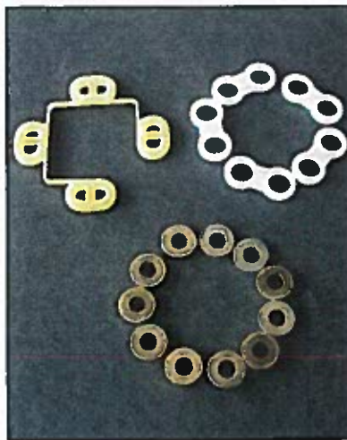
Photo 13 – Three styles of spacers used to center diaphragms in pump coil bodies. Original on all pumps (Healey BN1 – BJ8) is a set of 11 thick brass washers (bottom). The molded 4-part plastic spacer appeared on some replacement pumps in the 1980s and 1990s. This style works very well and is easy to install. The set of five figure 8 spacers is being supplied with pump rebuild kits today, and some of these spacers are too wide and will bind diaphragm operation. The brass rollers are tricky to install, but provide extremely dependable operation.
