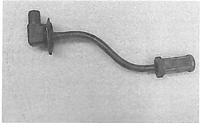
The pick-up tube removed from the fuel tank. The filter on the end of the pick-up tube cannot be changed since the pick-up tube cannot be removed except by cutting it out, damaging the fuel tank.
