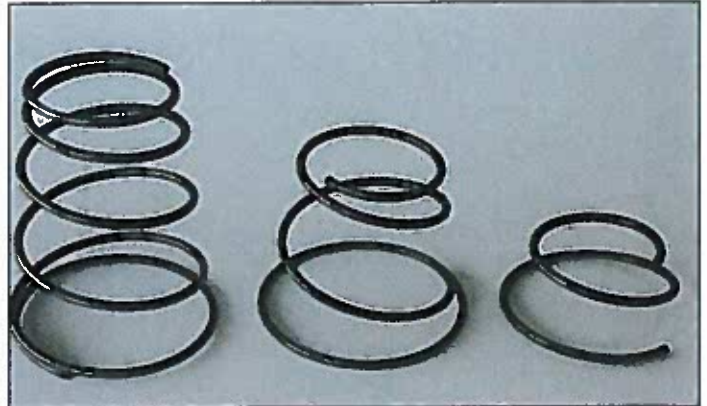
Photo 12 – The tall diaphragm spring on the left is used in HP pumps, found on Healey 100s. The middle spring was used on tall coil pumps in 100-Six and 3000 Healeys up to introduction of the short coil. The short spring on the right was only used with short coil pumps.
