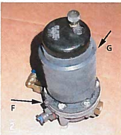
Photo 2 - The AUA 36 pump continued -- A screw (F) is available for attaching a grounding wire, though I've never seen this wire on original 100 pump installations. The boot (G) has writing molded into it. Note the molded writing on the flat cap. Original caps have a 12V molded in next to the terminal, as seen here. Flat caps were used on all pumps up to the last pump version [AUF 301] introduced in August, 1964 during early Phase 2 BJ8 production.
