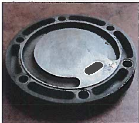
Photo 16 – A special gasket seals between this plate and the main pump body in AUA 36/56 pumps, and a second one against the pump diaphragm.
