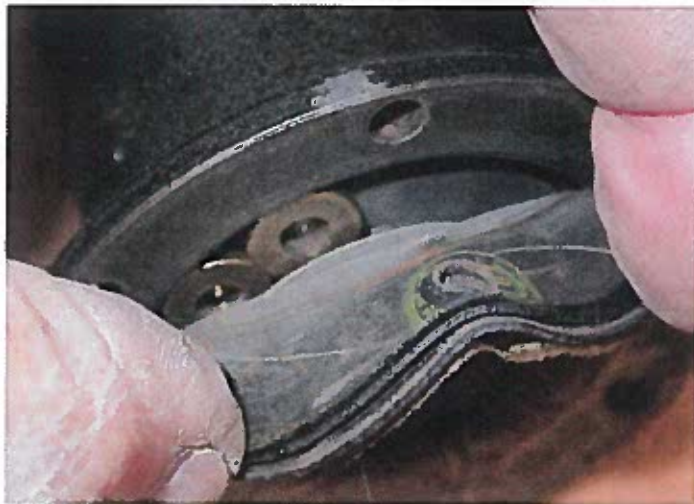
Photo 14 – Inserting the eleven rollers is tricky. You need to 1) make sure they seat properly into the metal diaphragm plate, 2) keep from falling out, and 3) insure that the diaphragm rotational alignment is not changed.
