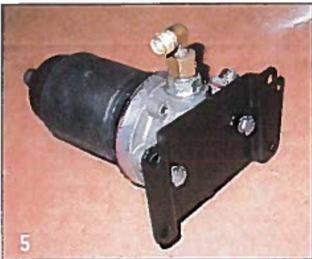
Photo 5 -- The AUA 56 pump was mounted to a shallow bracket using 1/4 BSF x 1/2 inch long hex screws. This bracket mounts to the rear axle side of the heel board behind the left seat.
