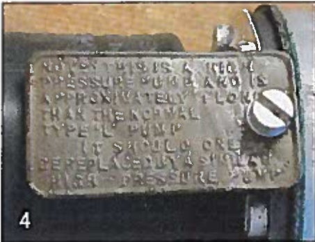
Photo 4 -- A pressed steel tag (also seen in Photo 3) has been found on some AUA 36 pumps, though it is not known whether these were used on many 100s. It identifies them as HP pumps.
