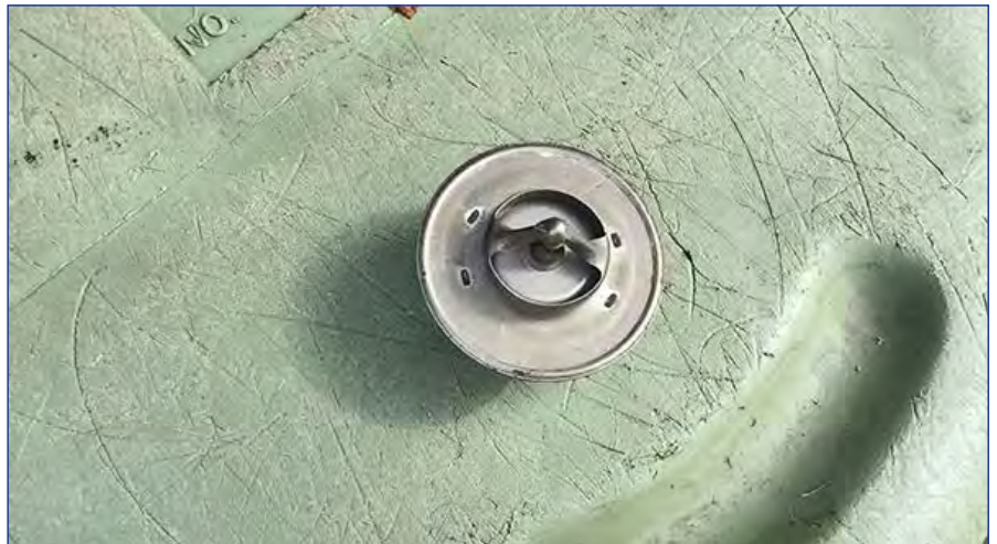
The bottom of the thermostat. As the engine heats up, the bottom of the thermostat elongates and pulls the thermostat open so coolant can flow.
