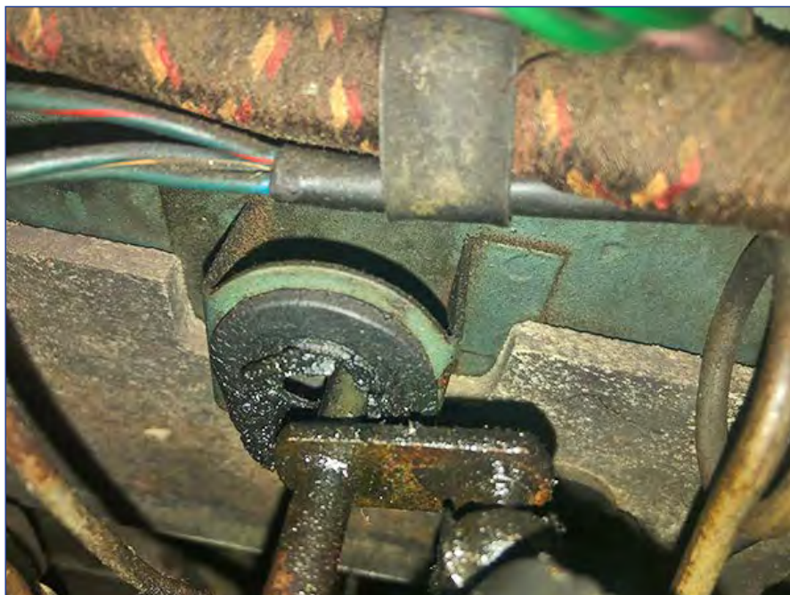
Throttle linkage shaft where it meets the firewall bushing. Note the rubber grommet around the bushing has perished.
