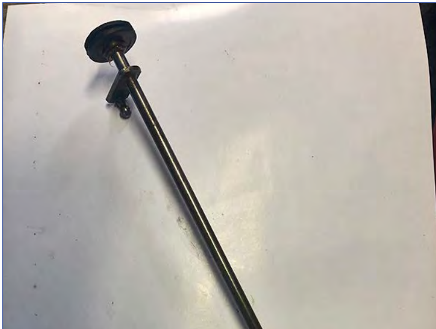
The throttle linkage shaft with the rubber grommet bushing and nylon bushing in their relative positions.
