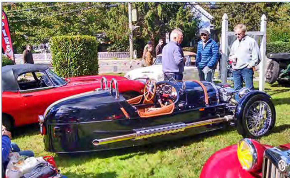
Modern replica of 1930s Morgan 3-wheeler, which had a motorcycle engine in the front.
