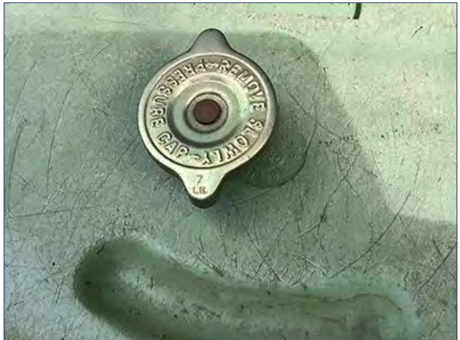
The Healey radiator pressure cap. You should be able to make out the number 7. All pressure caps have the pressure indicated on the top of the cap.
