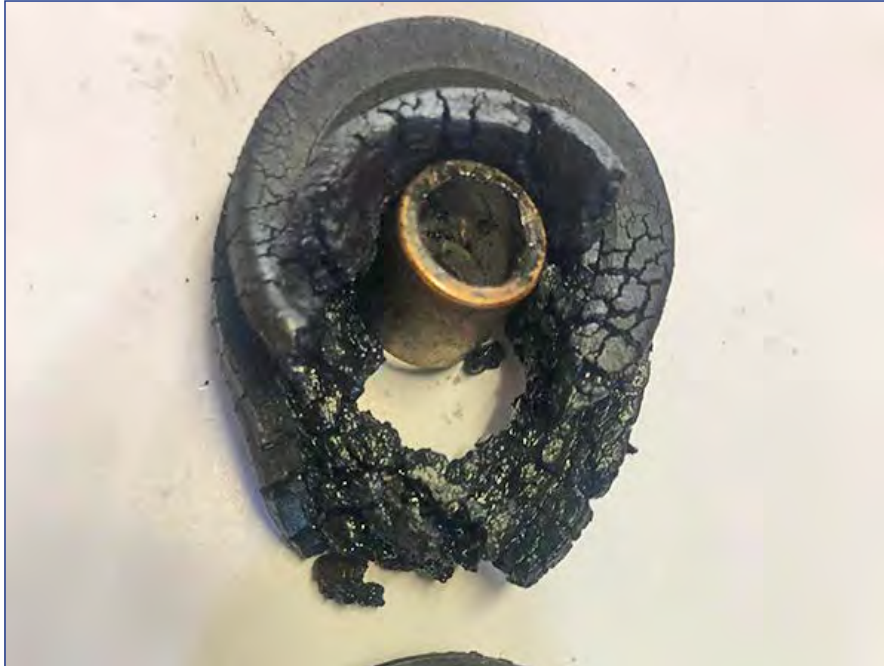
Old and new firewall grommet / bushing comparison. Replacement was overdue.
