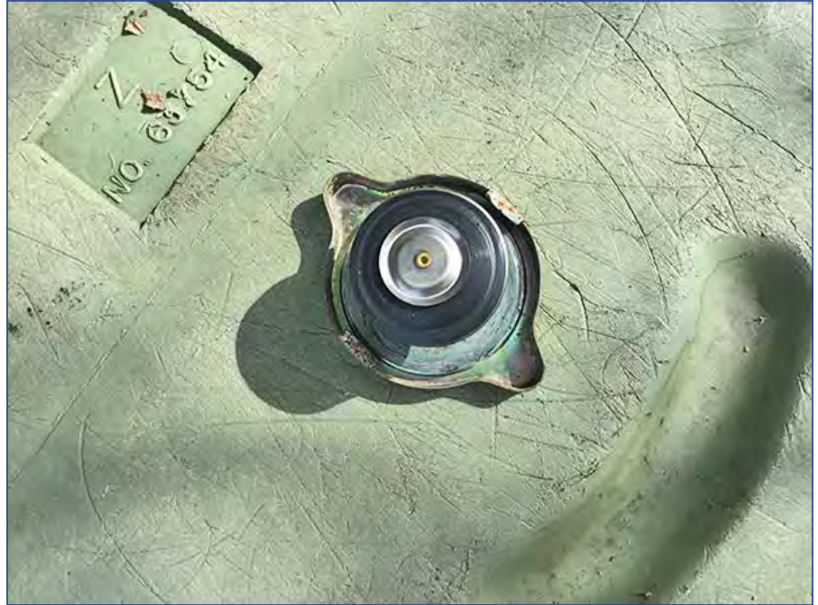
The Healey radiator pressure cap in my BJ8. This shows the part that goes in the radiator neck. The middle gasket with the rubber around it is the pressure valve, and the sealing of the cap is the silver-colored part around the outside,
