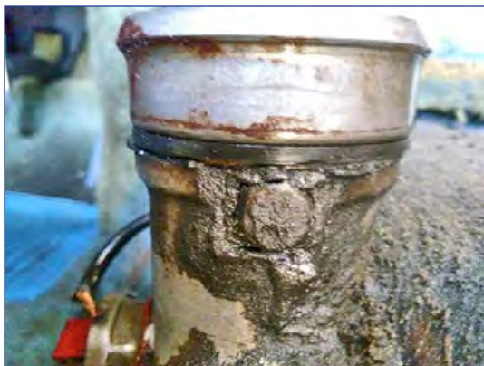
Shift lever retaining bolt, located at the 6 o'clock position, just below the cleaned up retaining cup.
