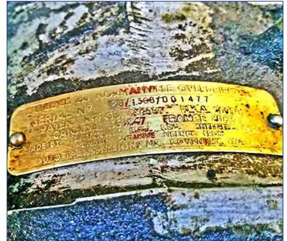
Brass ID plate for OD states "LAYCOCK de NORMANVILLE OVERDRIVE UNIT" with serial number 28/1308/001477.vv
