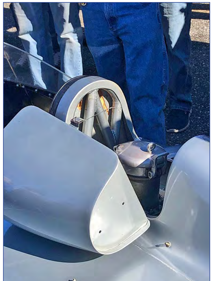
D type jag fin hatch open. Note the roll bar in the headrest and the fuel filler inches behind the driver's head! Blue 11 pts.
